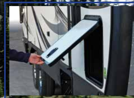
1" Thick Thermal Insulated Luggage Door Compartments
